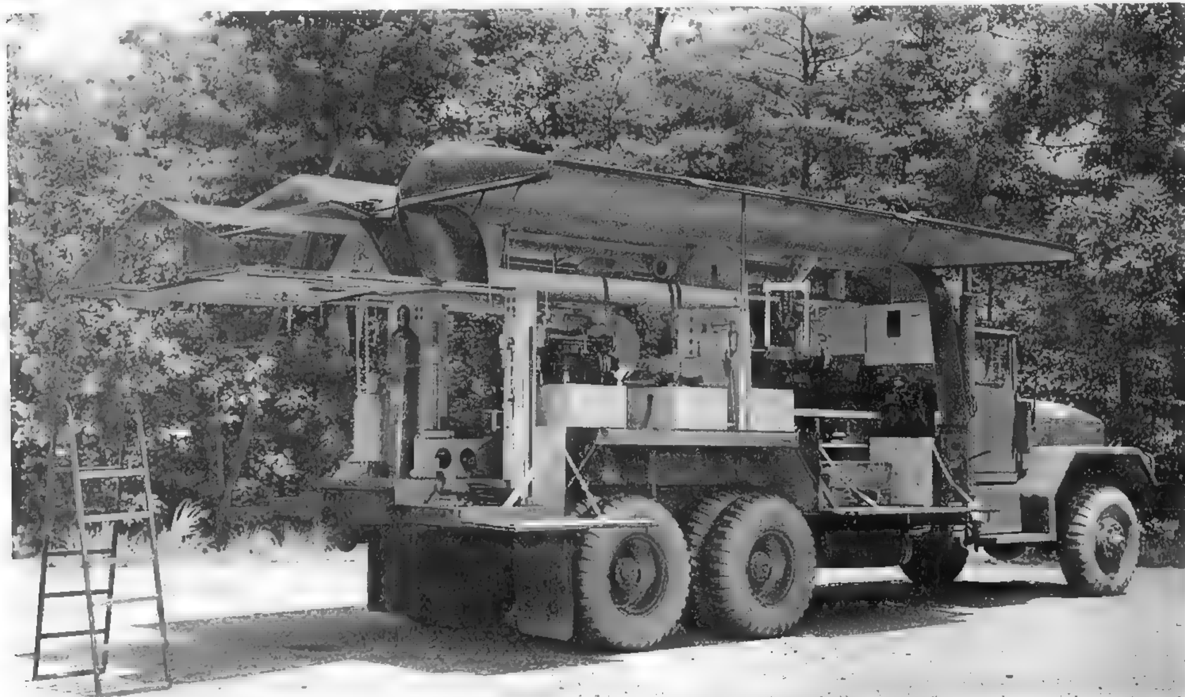
The mobile machine shop, having been deemed too heavy for the G-742 chassis, was mounted on the G-744, which was much better suited for the heavy load. (Photo courtesy of United States Army Engineer School History Office)
